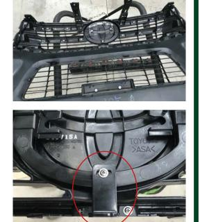
10. Once bull bar is aligned with vehicle and tightened, drill through pinning holes (circled in red) between bull bar and chassis bracket and secure with bolts, washers and nuts provided.
